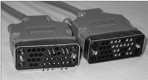
Figure 4-5 V.35 DTE and DCE Cables
